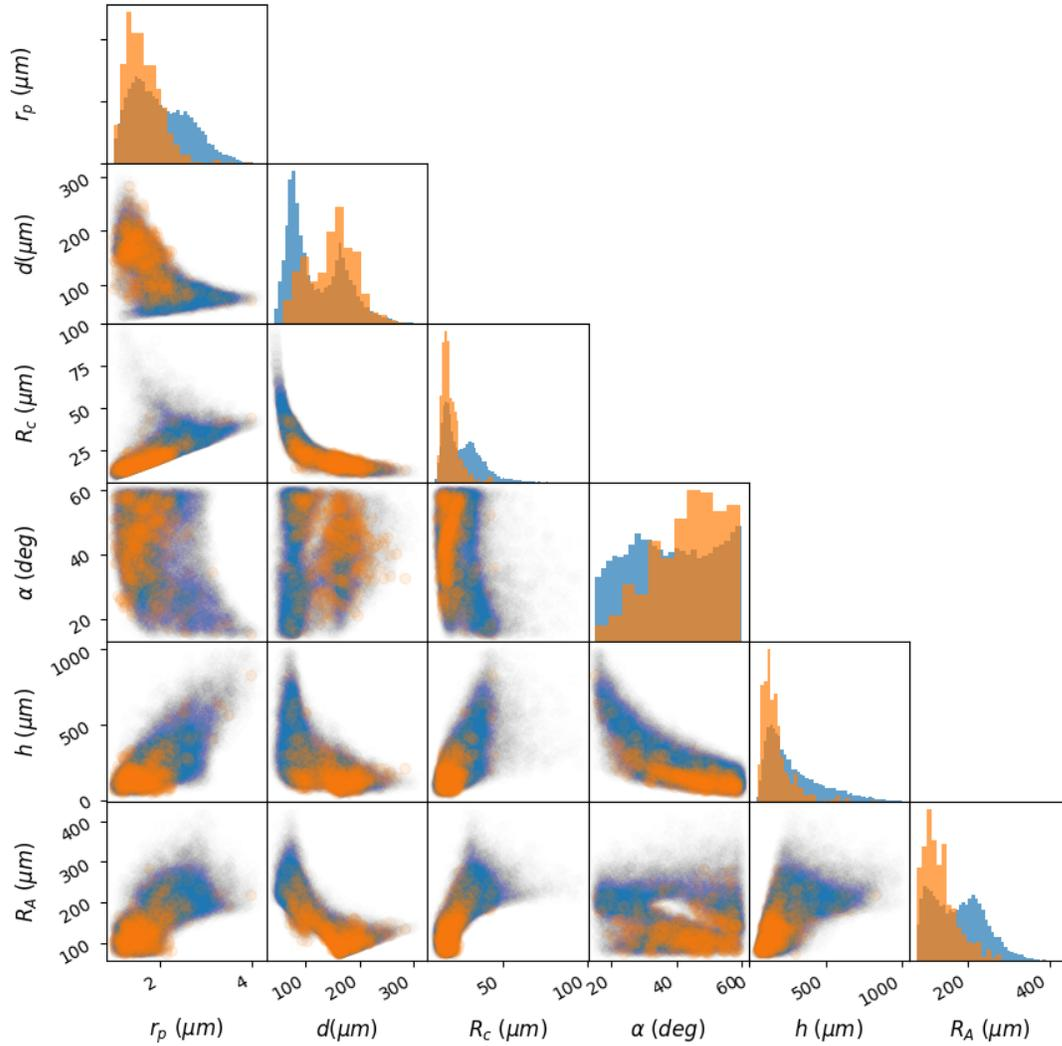
**Fig. 3** Comparison of designs satisfying deterministic (blue) and robust (orange) feasibility conditions. Diagonal plots show normalized histograms of the corresponding design variables sampled by the specified procedure. Off-diagonal plots show pair-wise designs. Deterministic designs often have bimodal and heavy-tailed behavior. Robust designs either fully or partially get rid of the bimodality, they also reduce the tails and concentrate in smaller regions.
