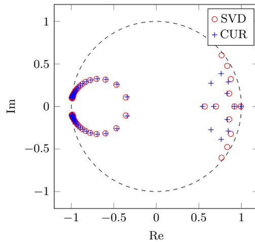
FIG. 1. Eigenvalues of the identified system matrix  $A_r$  via CUR-ERA and SVD-ERA, respectively.
