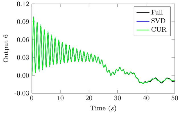
FIG. 5. Output No. 6 of the continuous-time systems realized using the full and the two identified reduced-order models.
