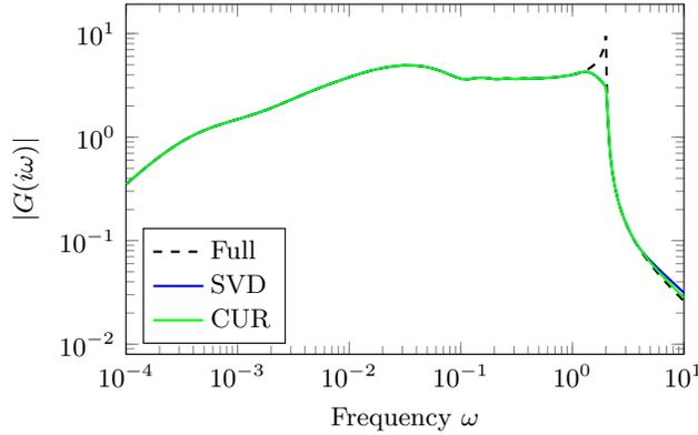
FIG. 3. Transfer function of the full model and the two reduced-order models identified from CUR-ERA and SVD-ERA.
